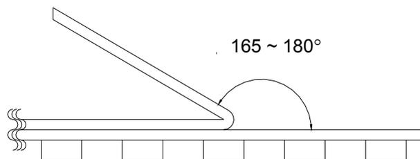
Fig.2. Taping Specification
