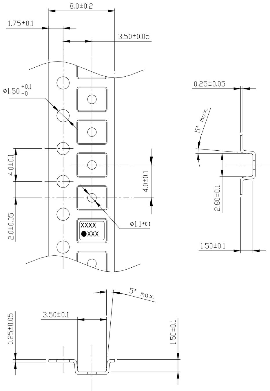
1) Clearance of an embossing tape, and a product unit : mm
